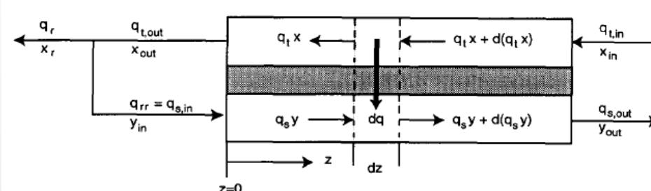
Fig. 3. Material balance for a permeator.
