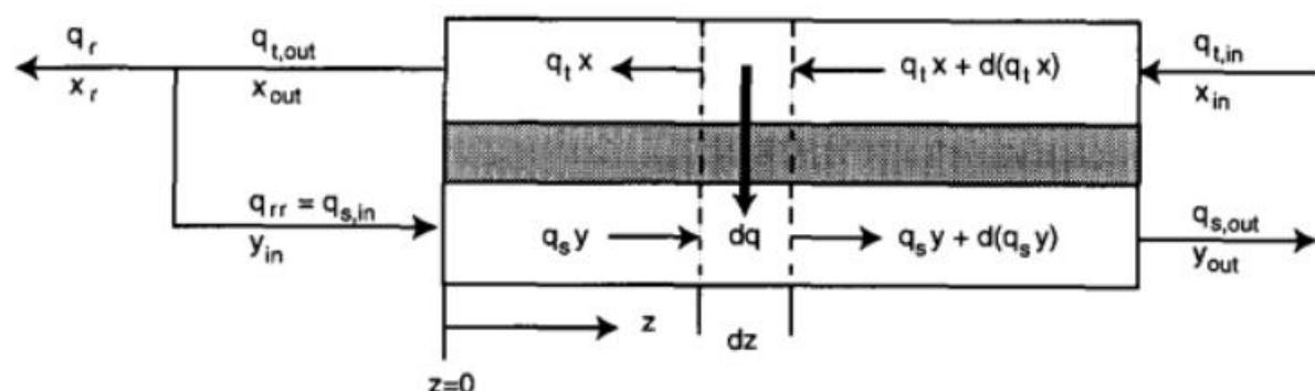
Fig. 3. Material balance for a permeator.
