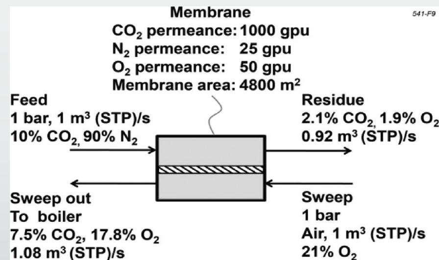
$$\text{Sweep ratio} = \frac{\text{Inlet sweep flow rate (m}^3\text{(STP)/s)}}{\text{Inlet feed flow rate (m}^3\text{(STP)/s)}}$$
