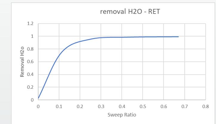
*Sweep mode : removal fraction increase with the sweep ratio*
