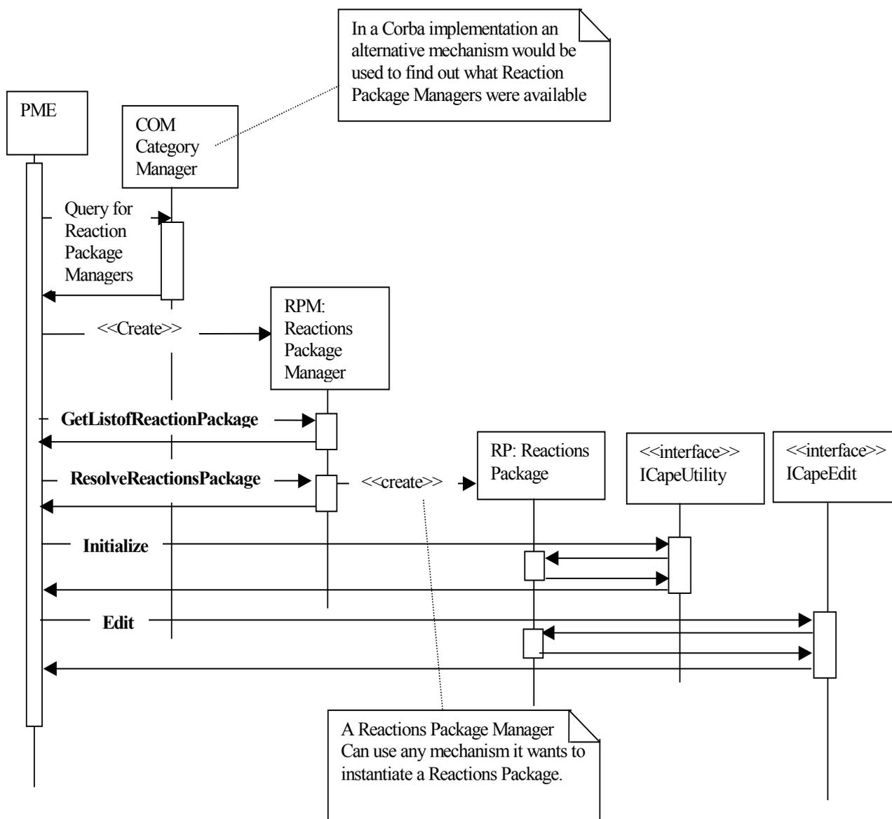
This sequence diagram shows the realisation of the following use cases in terms of the components and interfaces defined in this specification:
