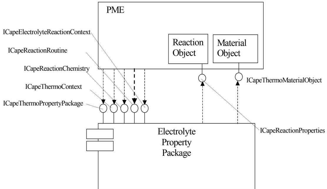
The following sequence diagram shows these interactions in more detail. Note that the next diagram is the same as the one for the interaction between a PME and a Reactions Package component, except that Reactions Package component is replaced by Electrolyte Property Package component. The Electrolyte package is able to perform its own thermodynamic Property calculations, and so does not rely on the PME to provide this service.
