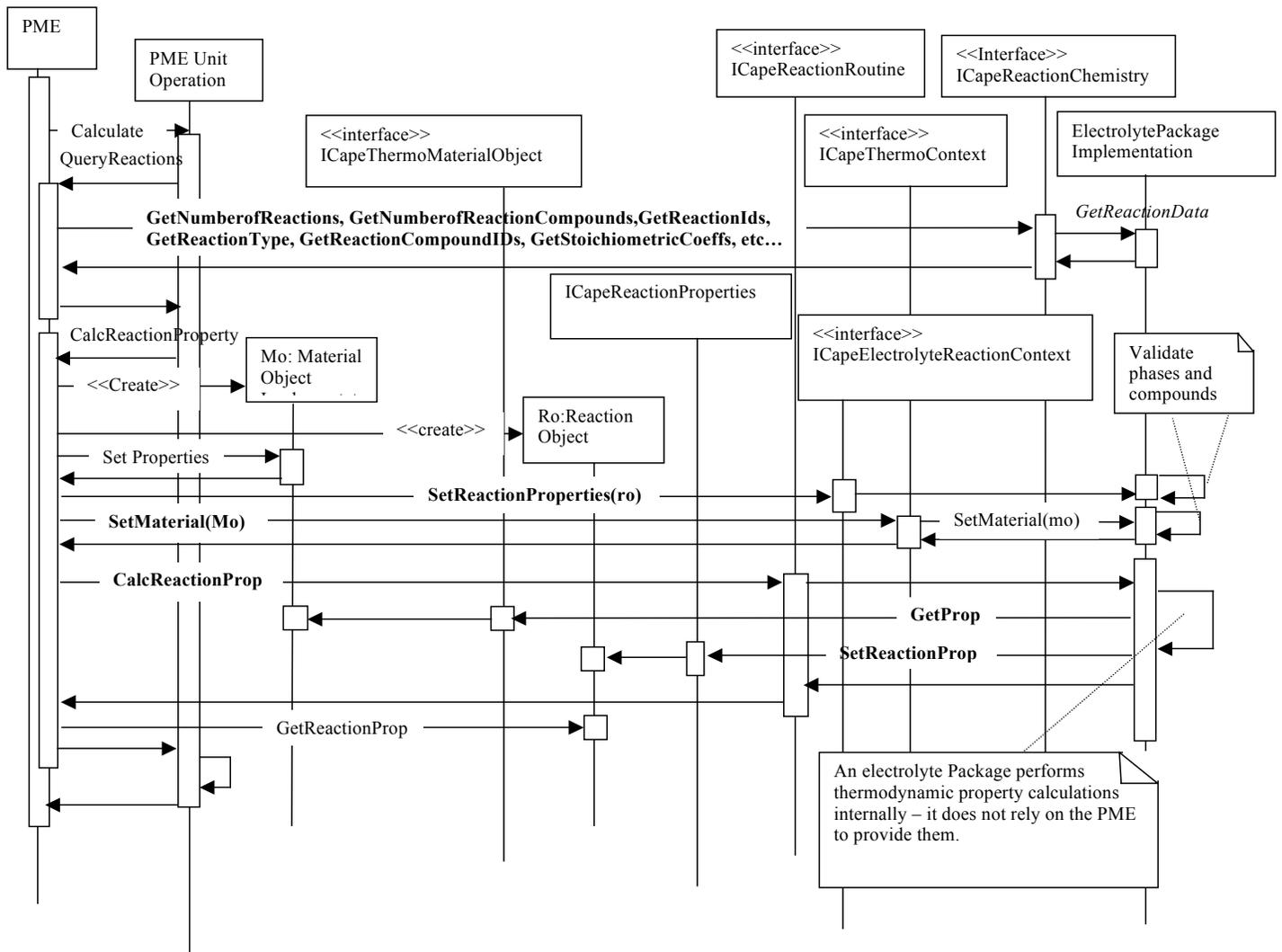
This sequence diagram shows the realisation of the following Use cases for the case of a set of electrolyte reactions:
