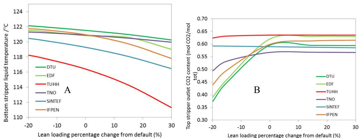
Fig. 8. (A) Outlet liquid temperature of the desorber bottom; (B) mole fraction of CO<sub>2</sub> in the stripped top gas.
