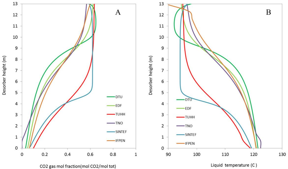
Fig. 12. Desorber CO<sub>2</sub> concentration profile (A) and liquid temperature profile for the case mentioned in table 3.
