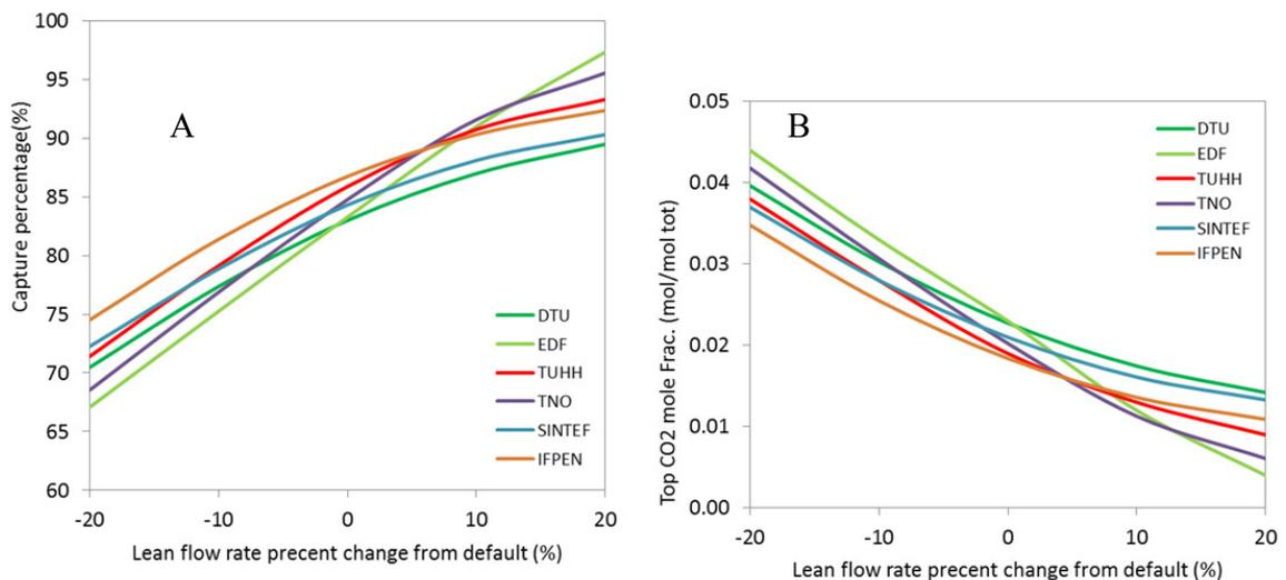
Fig. 2. (A) Absorber capture percentage; (B) absorber top gas phase mole fraction of CO<sub>2</sub> before washing.
