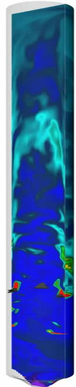
*MFIX validation and scale-up of a NCCC Transport Integrated Gasifier (gas temperature predictions of a commercial scale transport gasifier).*
